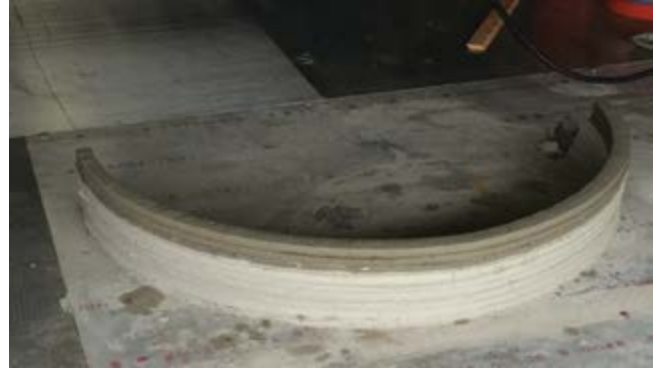
(a) Completed contour-crafted subscale straight wall segment and (b) subscale curved wall segment.
