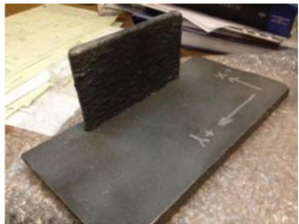
Figure 2: Typical MDDM Inconel® 718 build-up.
