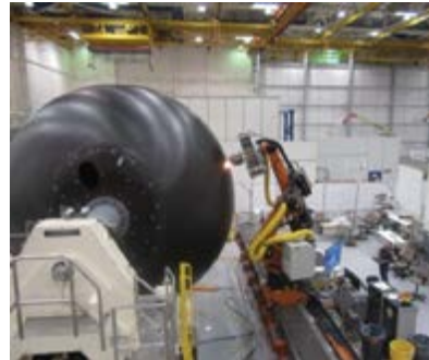
Figure 1: Fabrication of the 18-ft- (5.5-m-) all-diameter, all-composite tank at the Boeing facility.
