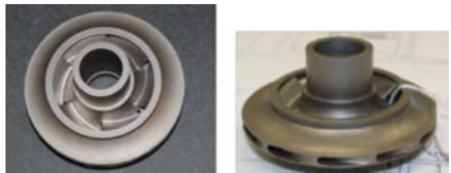
Figure 2: SLM Ti6-4 manufactured turbopump impeller.
