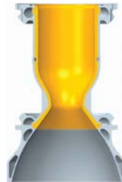
Chamber cross sections illustrating the copper alloy liner with built-in coolant passages and the deposited nickel alloy jacket and manifolds.
