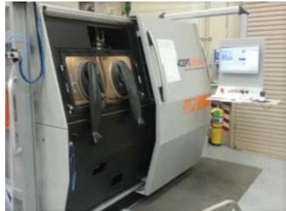
Figure 1: SLM machine with glovebox required for Ti64.
