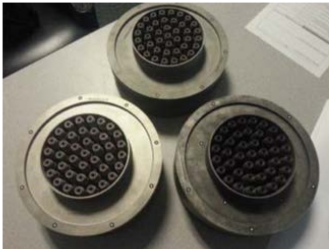
Figure 1: Manufactured liquid oxygen/hydrogen SLM injectors.
