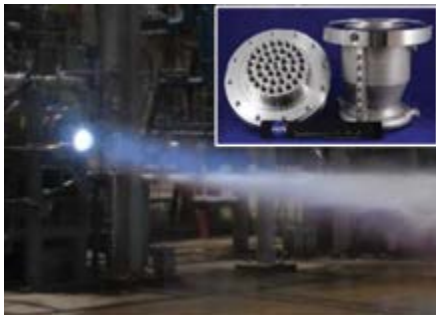
Figure 6: LOX/LCH 4 regenerative cool chamber hot-fire test.
