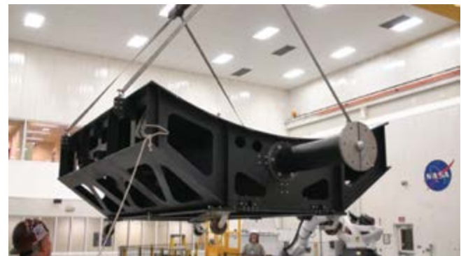
Figure 4: Composite tool manufactured by Janicki Industries.
