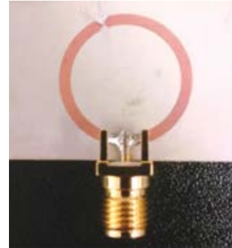
Figure 1: An SRR fabricated with photolithography. The SMA connector supplies the driving microwave power. The unseen backside of the white substrate is fully clad in copper and acts as the ground plane.
