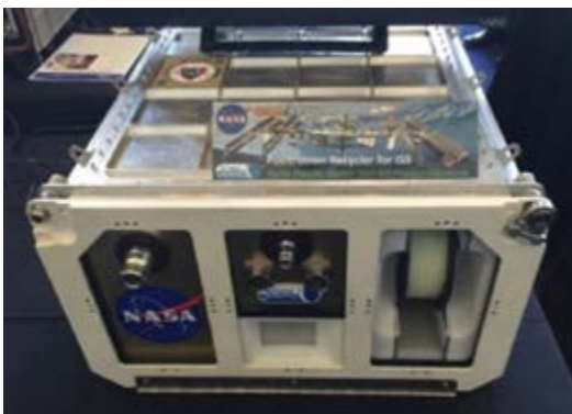
Figure 2: Recycler for on-orbit demonstration as part of Phase II SBIR to recycle 3D-printed parts back into feedstock.
