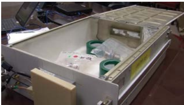
Figure 3: RFID-enabled ISIS drawer.
