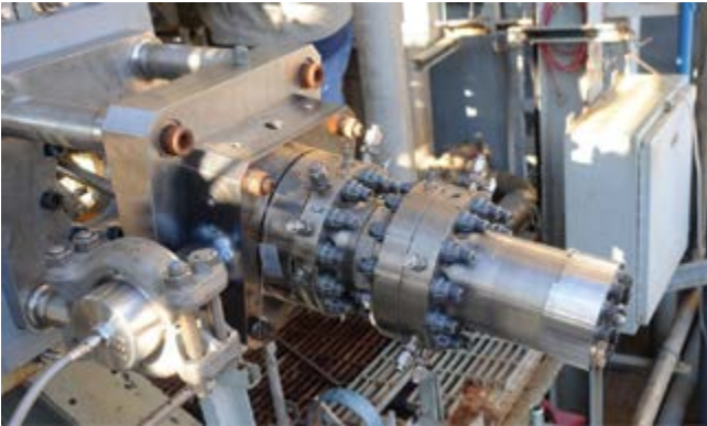
Figure 2: MSFC's oxygen-rich/RP-1 preburner assembly.
