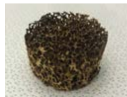
Figure 5: Iron coated on copper substrate using an ionic liquid.
