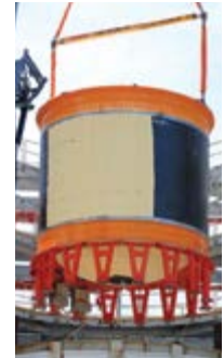
Figure 2: All-composite tank being tested at MSFC.
