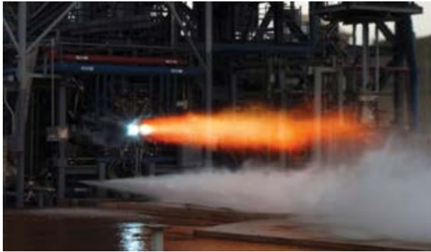
Example of a previous engine component testing at MSFC's Test Stand 116. LCUSP combustion chamber will be tested at similar liquid hydrogen and liquid oxygen flow rates and thrust levels.
