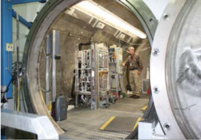
Integrated test chamber enables testing of LSS technologies in an environment that simulates human metabolic activity integrated with functional LSS hardware.
