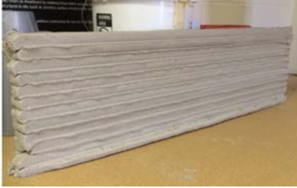
(a) Completed contour-crafted subscale straight wall segment and (b) subscale curved wall segment.
