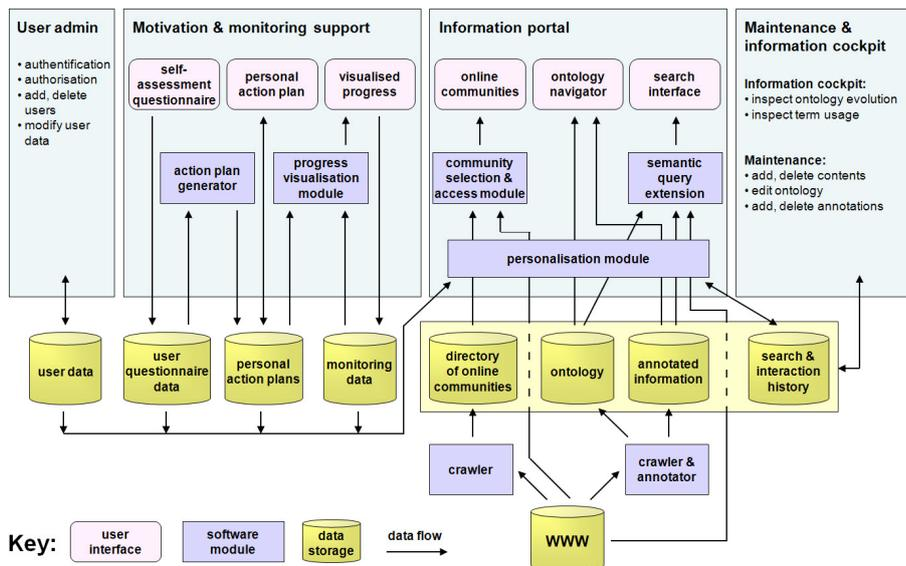
Fig. 1. System architecture of SEMPER
